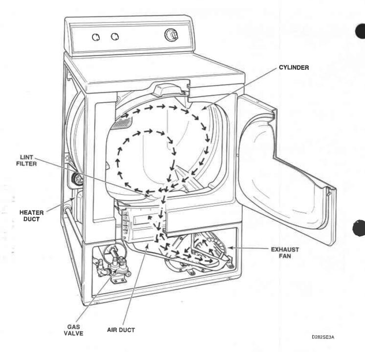
The dryer uses heated air to dry loads of laundry. When the motor is started, the exhaust fan pulls room temperature air in through louvers at the rear of the dryer and over the heat source (burner flame for gas and heating element for electric). The heated air moves through the air duct and into the cylinder, where it circulates through the wet load. The air then passes through the lint filter, exhaust fan, and is vented to the outdoors.
