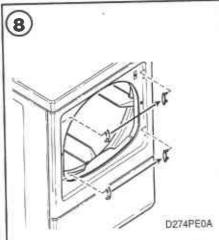
Using a screwdriver, remove two door plugs, and reinstall on opposite side of door opening.
