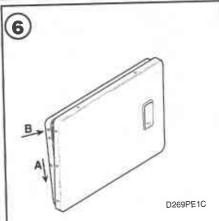
Insert liner under flange on bottom of door, then push top of door liner into place.
