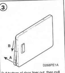
Pull bottom of door liner out, then pull down, removing door liner from door panel.
