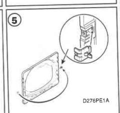
Remove door strike from door liner and reinstall on opposite side.
