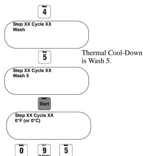
Enter desired temperature for load to cool down to. Three digits must be used for temperature. If Fahrenheit, the valid temperature range is  $80^{\circ} - 200^{\circ}$ F. If Celcius, valid temperature range is  $25^{\circ} - 90^{\circ}$ C (example:  $95^{\circ}$ F).
