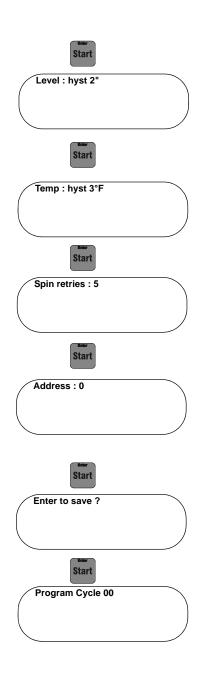
Press "Enter" to set the hysteresis level (level at which water drops before it senses it must refill).
