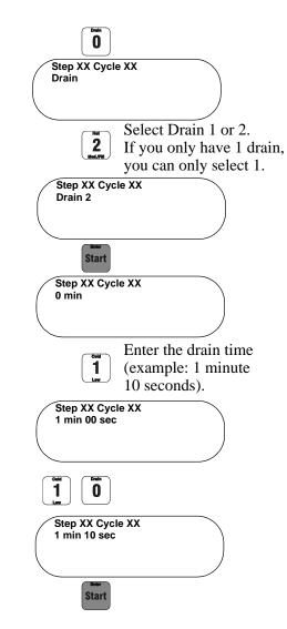
NOTE: With the WE-8 control, it is NOT necessary to program a drain step before spin. The spin step incorporates the balancing routine and draining before beginning high speed spin (as a sub part of the spin step). A programmed drain step will be skipped if spin step is programmed immediately after it.
