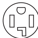
4-wire receptacle (14-30R)
