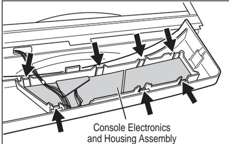
**Figure 19.** Locate seven locking tabs.
