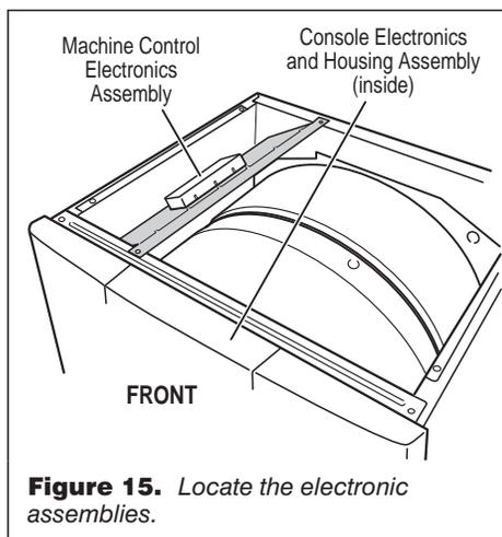
**Figure 15.** Locate the electronic assemblies.
