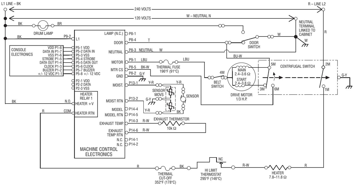
**GAS DRYER WIRING DIAGRAM**
