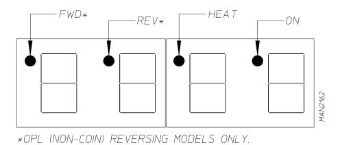
d. Verify that motor(s) heat, and door indicator lights on the back side of the microprocessor (computer) board are lit. (Refer to illustration below.)
