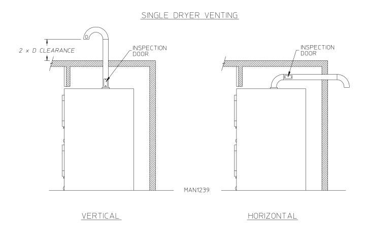
**IMPORTANT: DO NOT** use screens or caps on the outside opening of exhaust duct work.
