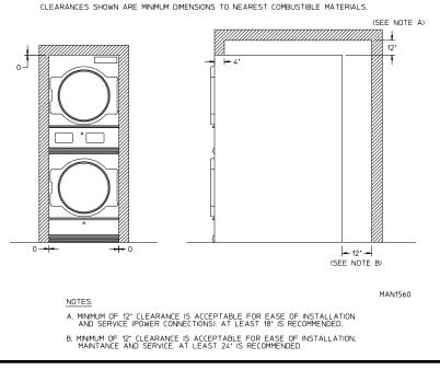
**IMPORTANT:** Dryer *should be* located where a minimum amount of exhaust duct *will be* necessary.
