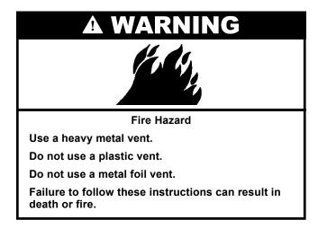
As per the National Fuel Gas Code, "Exhaust ducts for type 2 clothes dryers shall be constructed of sheet metal or other noncombustible material. Such ducts shall be equivalent in strength and corrosion resistance to ducts made of galvanized sheet steel not less than 26 gauge (0.0195-inches [0.50 mm]) thick."
