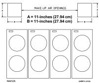
EXAMPLE: For a bank of 4 dryers, 2 unrestricted openings measuring 11-inches by 11-inches (27.94 cm by 27.94 cm) are acceptable.
