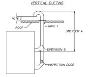
NOTE 1 Opening from combustible materials must be 2-inches (5.08 cm) larger than the duct (all the way around). The duct must be centered within this opening.
