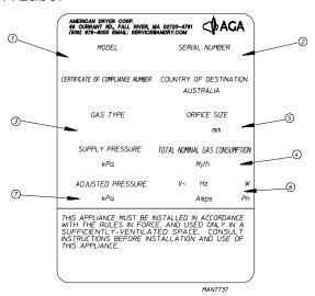
When contacting ADC, the information on the data label is required to ensure proper service/parts assistance. The data label is located at the upper left rear of the dryer behind the back guard.
