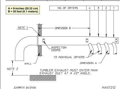
NOTE 1 Opening must be 2-inches (5.08 cm) larger than the duct (all the way around). The duct must be centered within this opening.
