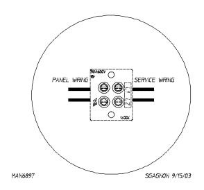
A ground lug is provided in the rear electrical box to connect your service ground.
