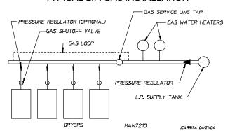
Consistent gas pressure is essential at all gas connections. It is recommended that a 3/4-inch (19.05 mm) pipe gas loop be installed in the supply line servicing a bank of dryers. An in-line pressure regulator must be installed in the gas supply line (header) if the (natural) gas pressure exceeds 12.0 inches (29.9 mb) of W.C. pressure.
