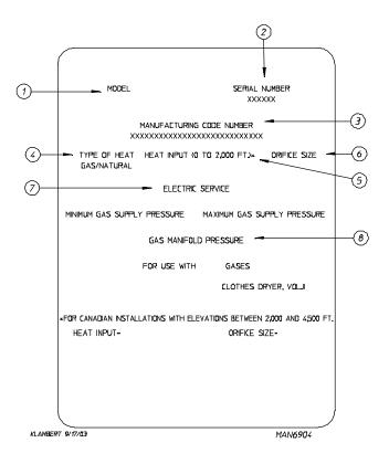
When contacting ADC, certain information is required to ensure proper service/parts information from ADC. This information is on the data label affixed to the left side panel area behind the top control (access) door. When contacting ADC please have the model number and serial number available.
