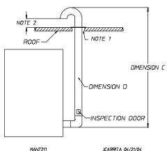
NOTE 1 Opening must be 2-inches (5.08 cm) larger than the duct (all the way around). The duct must be centered within this opening.
