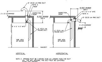
If the length of the duct run or quantity of elbows used exceeds the above noted specifications, the cross-sectional area of the ductwork may need to be increased.
