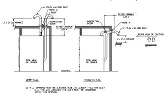
If the length of the duct run or quantity of elbows used exceeds the above noted specifications, the cross-sectional area of the ductwork may need to be increased.
