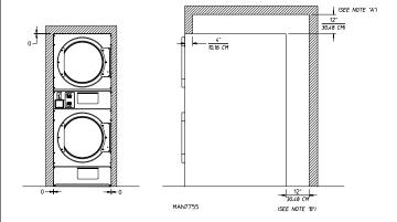
NOTE A: 12-inch (30.48 cm) minimum, 18-inches (45.7 cm) is suggested for ease of maintenance.
