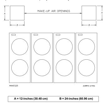
EXAMPLE: For a bank of 4 dryers, 2 unrestricted openings measuring 12-inches by 24-inches (30.48 cm by 60.96 cm) are acceptable.
