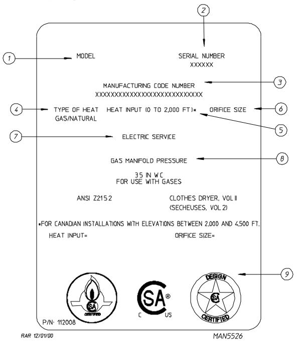
When contacting **ADC**, certain information is required to insure proper service/parts information from **ADC**. This information is on the dryer data label affixed to the back panel of the main electrical cabinet located in the right hand electrical enclosure. When contacting **ADC** please have the <u>model number</u> and <u>serial number</u> available.
