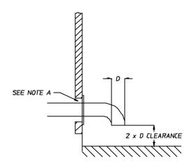
NOTE "A" OPENING MUST BE TWO (2) INCHES (5.08 CM) LARGER THAN DILCT (ALL THE MAY AROUND). THE DUICT MUST BE CENTERED WITHIN THIS OPENING
