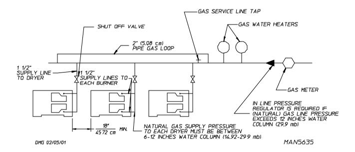
Consistent gas pressure is essential at <u>ALL</u> gas connections. <u>It is recommended</u> that a 2-inch (5.08 cm) pipe gas loop be installed in the supply line servicing a bank of dryers. An in-line pressure regulator **must be** installed in the gas supply line (header) if the (natural) gas pressure exceeds 12.0 inches (29.9 mb) of water column (W.C.) pressure.
