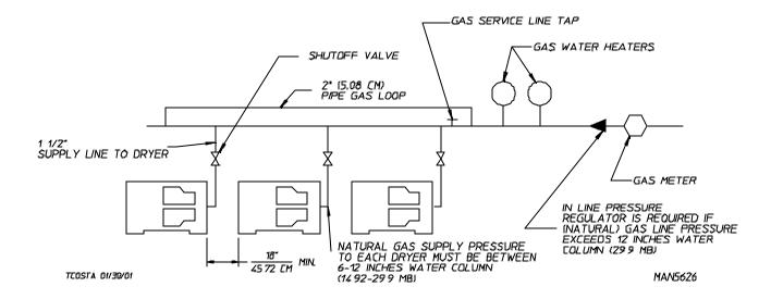
Consistent gas pressure is essential at <u>ALL</u> gas connections. <u>It is recommended</u> that a 2-inch (5.08 cm) pipe gas loop be installed in the supply line servicing a bank of dryers. An in-line pressure regulator **must be** installed in the gas supply line (header) if the (natural) gas pressure exceeds 12.0 inches (29.9 mb) of water column (W.C.) pressure.
