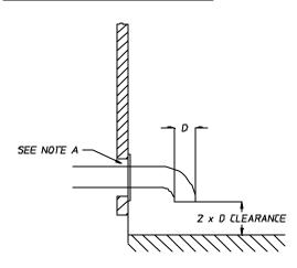
NOTE "A" OPENING MUST BE TWO (2) INCHES (5.08 CM) LARGER THAN DILCT (ALL THE MAY AROUND). THE DUICT MUST BE CENTERED WITHIN THIS OPENING
