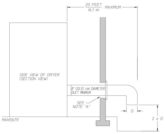
NOTE A: OPENING MUST BE 2-INCHES (5.08 cm) LARGER THAN THE DUCT (ALL THE WAY AROUND).
