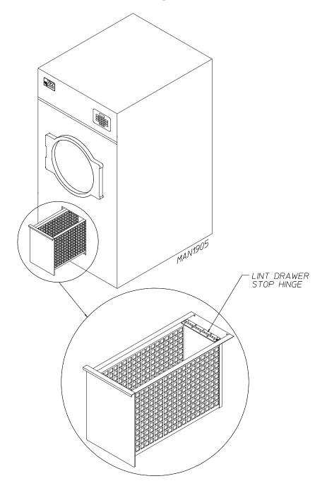
**IMPORTANT:** After replacing the lint drawer back into the dryer, be sure to rotate/move hinge back to the upward stop position.
