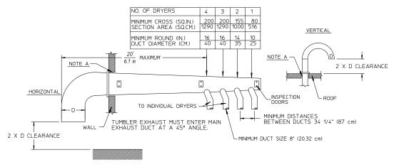
IMPORTANT: NO MORE THAN 4 DRYERS CAN BE CONNECTED TO ONE COMMON DUCT ( VENT ).
