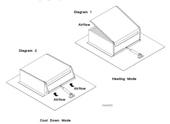
**NOTE:** With the dryer off or with no air supply, the steam damper is in cool down mode as shown in Diagram 2.
