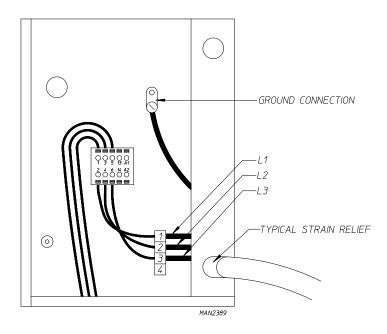
Providing local codes permit, power to a gas dryer or steam dryer can be made by the use of a flexible U.L. listed power cord or pigtail (wire size **must conform** to rating of dryer), or the dryer can be hard wired directly to the service breaker panel. In <u>ALL</u> cases, a strain relief **must be** installed where the wiring enters the dryer and service box area.
