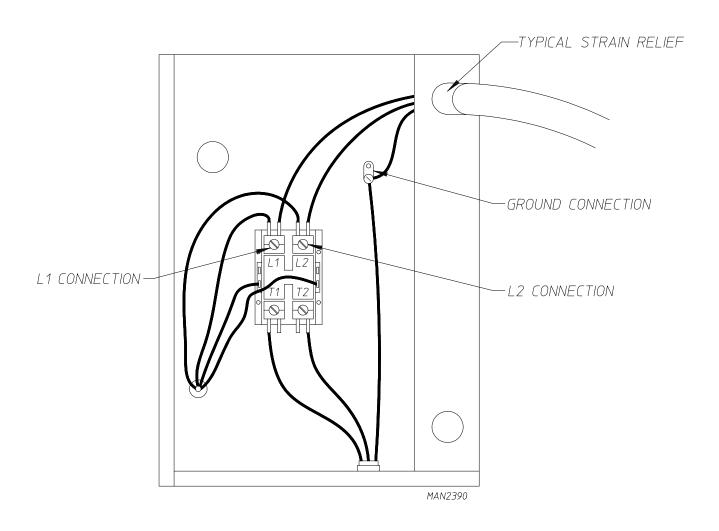
If local codes permit, power to the dryer can be made by the use of a flexible U.L. listed power cord or pigtail (wire size **must conform** to rating of dryer), or the dryer can be hard wired directly to the service breaker panel. In both cases, a strain relief **must be** installed where the wiring enters the dryer.
