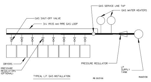
Consistent gas pressure is essential at <u>ALL</u> gas connections. <u>It is recommended</u> that a 3/4-inch (19.05 mm) pipe gas loop be installed in the supply line servicing a bank of dryers. An in-line pressure regulator **must be** installed in the gas supply line (header) if the (natural) gas pressure exceeds 12.0 inches (29.9 mb) of water column (W.C.) pressure. (Refer to the illustrations on the previous page.)
