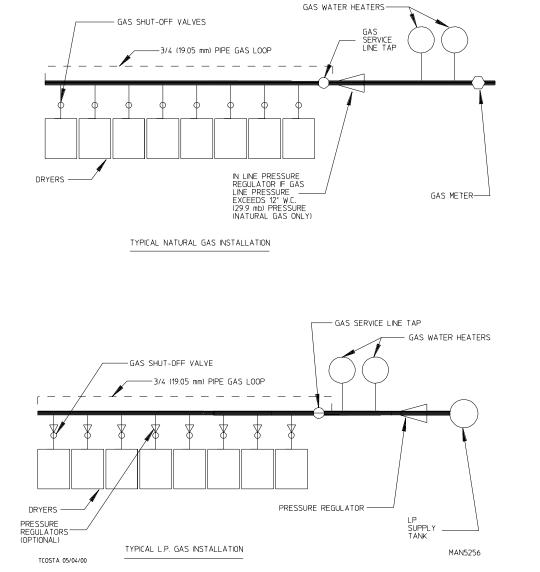
Consistent gas pressure is essential at <u>ALL</u> gas connections. <u>It is recommended</u> that a 3/4-inch (19.05 mm) pipe gas loop be installed in the supply line servicing a bank of dryers. An in-line pressure regulator **must be** installed in the gas supply line (header) if the (natural) gas pressure exceeds 12.0 inches (29.9 mb) of water column (W.C.) pressure. (Refer to the **illustrations** on the previous page.)
