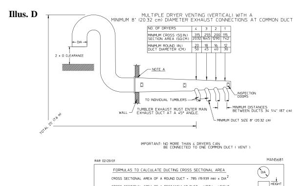
NOTE A: OPENING MUST BE 2-INCHES (5.08 cm) LARGER THAN THE DUCT (ALL THE WAY AROUND). THE DUCT MUST BE CENTERED WITHIN THIS OPENING.
