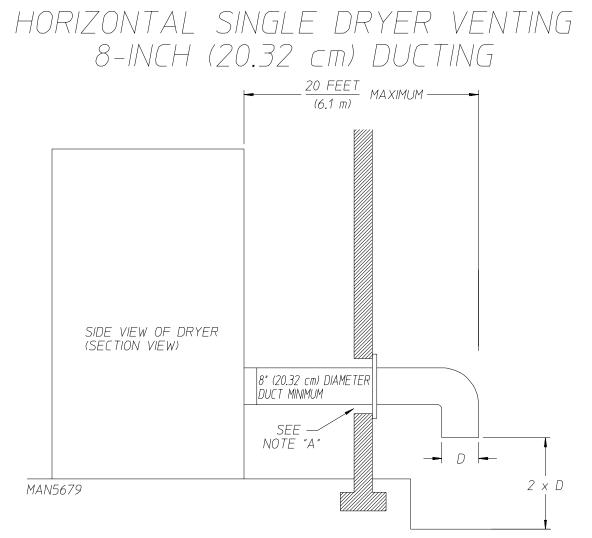
NOTE A: OPENING MUST BE 2-INCHES (5.08 cm) LARGER THAN THE DUCT (ALL THE WAY AROUND). THE DUCT MUST BE CENTERED WITHIN THIS OPENING.
