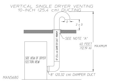
NOTE A: OPENING MUST BE 2-INCHES (5.08 cm) LARGER THAN THE DUCT (ALL THE WAY AROUND). THE DUCT MUST BE CENTERED WITHIN THIS OPENING.
