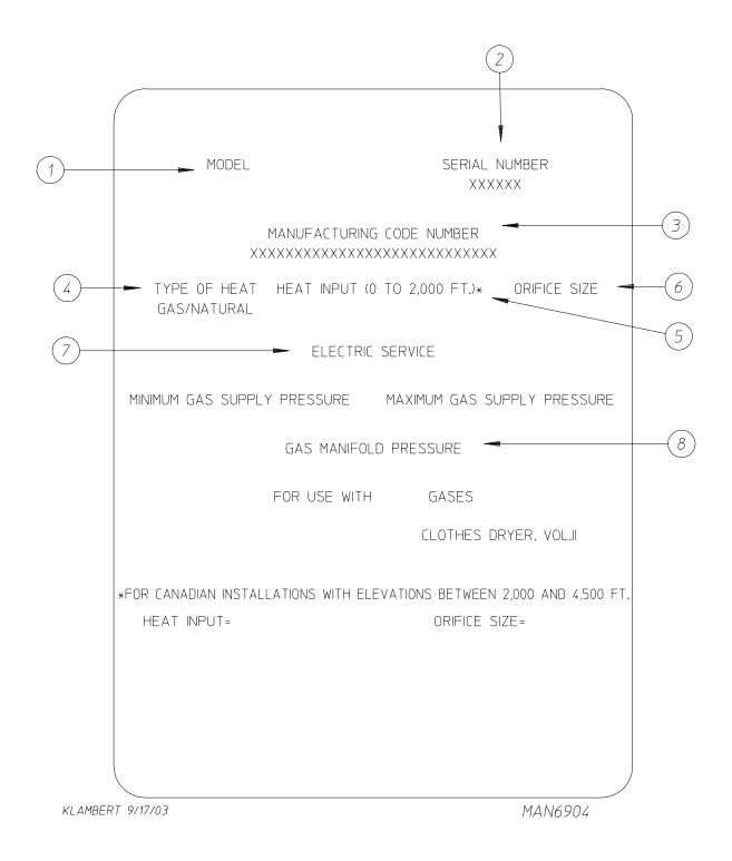
When contacting **American Dryer Corporation**, certain information is required to ensure proper service/parts information from **ADC**. This information is on the data label located on the left wall area behind the upper or top control door. When contacting **ADC**, please have the **model number** and **serial number** available.
