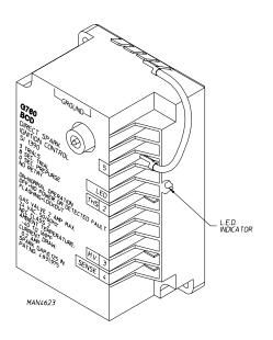
No L.E.D. indicator indicates a power or an internal failure has occurred.
