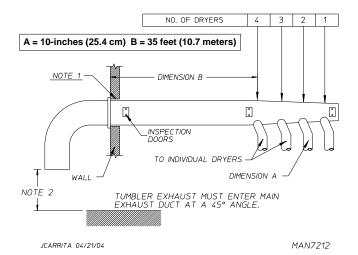
NOTE 1 Opening from combustible materials must be 2-inches (5.08 cm) larger than the duct (all the way around). The duct must be centered within this opening.
