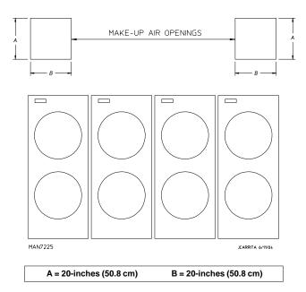
EXAMPLE: For a bank of 4 dryers, 2 unrestricted openings measuring 20-inches by 20-inches (50.8 cm by 50.8 cm) are acceptable.
