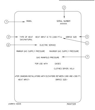
When contacting ADC, certain information is required to ensure proper service/parts information from ADC. This information is on the data label affixed to the right side panel area at the rear of the dryer. When contacting ADC, please have the model number and serial number available.
