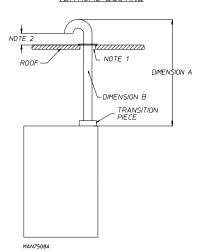
NOTE 1 Opening from combustible materials must be 2-inches (5.08 cm) larger than the duct (all the way around). The duct must be centered within this opening.
