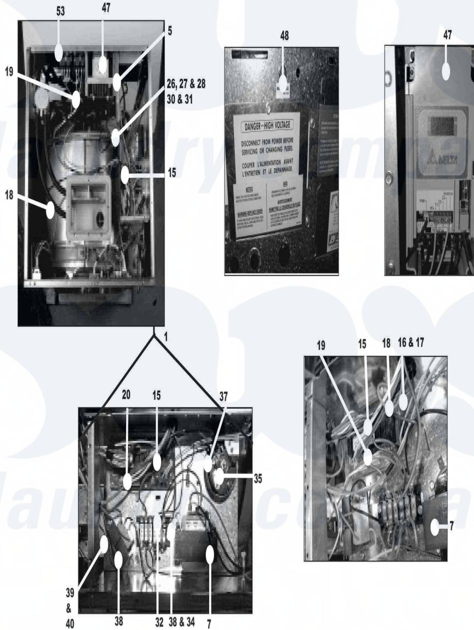
Dexter Commercial Dexter WCAD18KCS-12 (T-300) Washer Parts Parts Diagram Electrical Components
