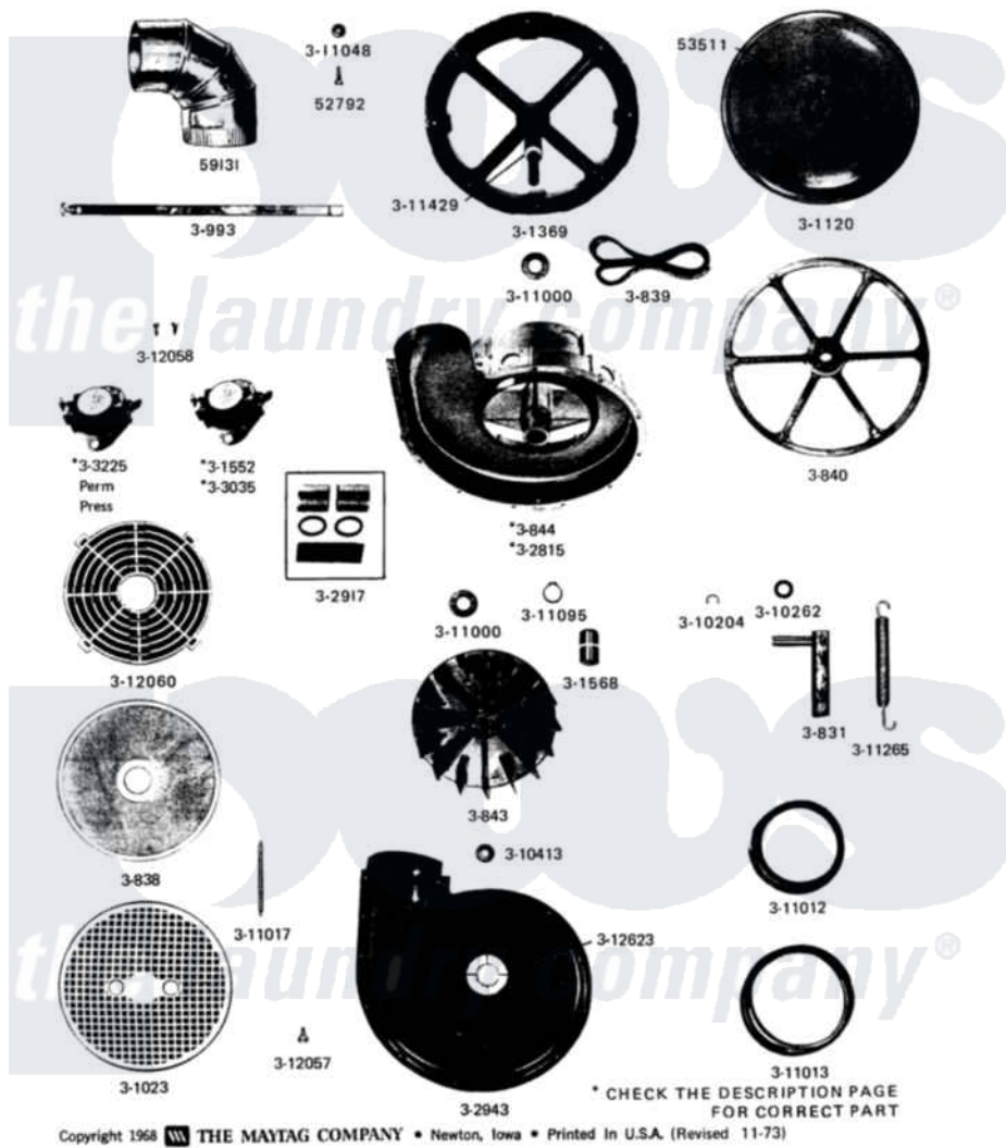
Maytag Residential Maytag DG16CA Dryer Parts Parts Diagram 07 - EXHAUST & BLOWER ASSEMBLY Click on the part number to view part
