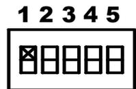
1. Activate the Bill Acceptance and/or Bill Acceptance Security Level mode by setting: Switch 1–ON; Switch 2–OFF; Switch 3–OFF; Switch 4–OFF; Switch 5–ON
