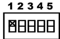
1. Activate the No Coin Acceptor Shutdown programming mode by setting:
