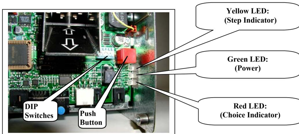
**Step Indicator** - The yellow or top LED is the *Step indicator*. During the programming sequence, this LED flashes a code indicating which *Step* you are on or when flashing in unison with the red LED indicating which group you are in.
